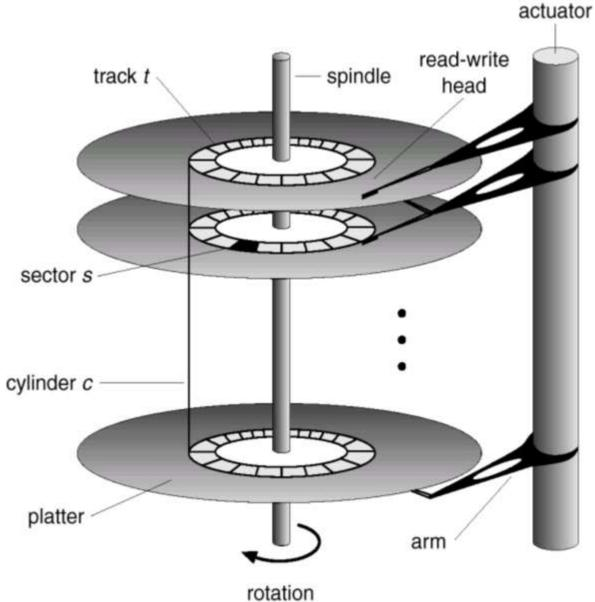
A single stepper motor controls all the heads, so all heads move together.
