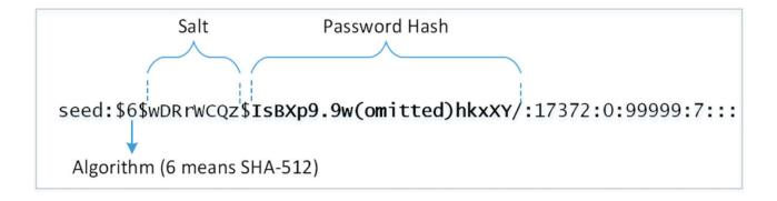
Every row contains one record having nine colon separated fields. Here is the breakdown of each field: user:\$y\$salt\$hash:lastchanged:min:max:warn:inactive:expire:
