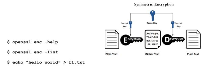
\$ openssl enc -des -in f1.txt -out encrypted\_des -K 0123456789abcdef -iv a0b0c1d4e5f27891
